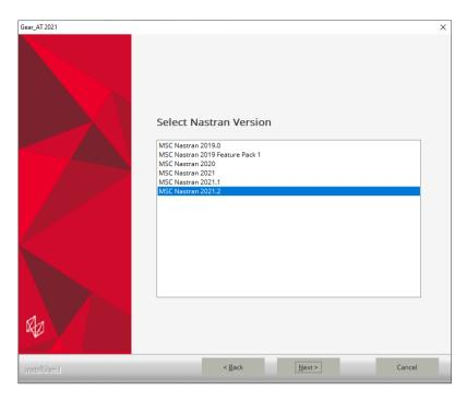
You can proceed with the installation of Gear AT without Nastran and install it later, but you have to set up NASTRAN\_TOP\_DIR environment variable manually. This variable should point to the Nastran installation directory, e. g. c:\MSC.Software\MSC\_Nastran\2021.2
