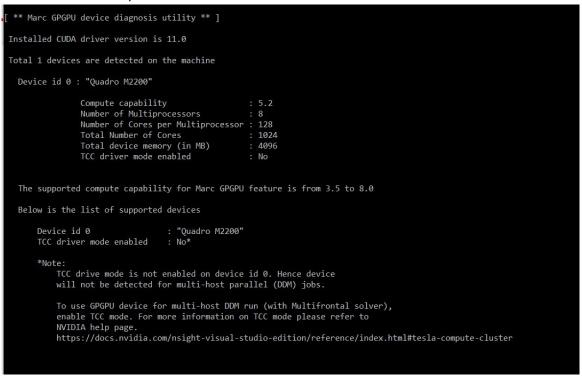
Figure 2-4 Deviceinfo.bat Output
