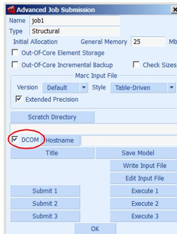
Figure 2-3 Advanced Job Submission Menu Displaying the DCOM Option
